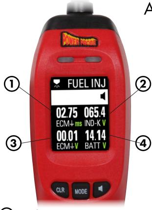
Advanced Testing Operations Fuel Injector Mode
