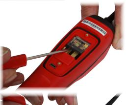
Using an appropriate pry tool or small screwdriver, carefully pry the Circuit Breaker towards the tip to dis-engage it from the breaker terminals. Do not apply excessive force.
