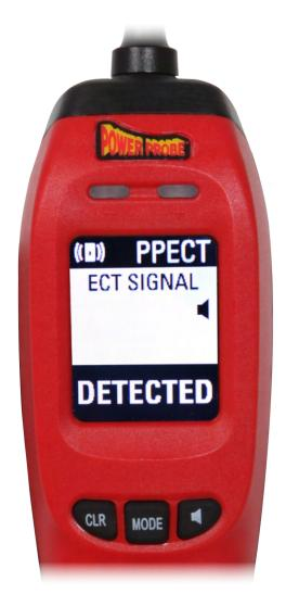
(1) **PPECT** = PPECT Mode is designed to work with the Power Probe ECT2000 for locating open circuit conditions in wiring.
