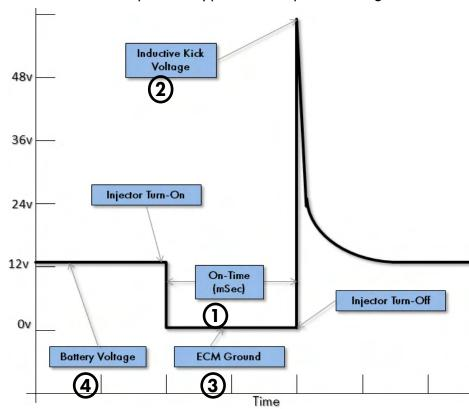
a single injector pulse. The vertical axis represents the circuit voltage and the horizontal axis represents time.
